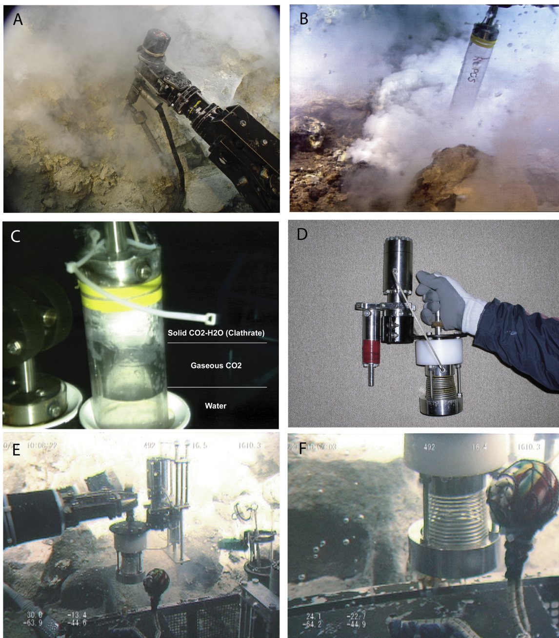
Figure 6. Photographs of sampling at the Champagne site in 2004 and 2005. (a) Fluid sampler being inserted into 103°C hydrothermal vent. (b) Droplets of liquid CO 2 being collected in an inverted plastic cylinder held in the ROV arm. (c) Photograph of the plastic cylinder taken at about 400 m depth during the ROV’s ascent to the surface. Most of the liquid droplets have converted to hydrate, and the hydrate is beginning to sublime into gaseous CO 2 . (d) Close-up of the “droplet catcher” used during the 2005 expedition attached to the small volume gas-tight bottle. (e and f) The ROV Hyper-Dolphin sampling liquid CO 2 with the droplet catcher and gas-tight bottle at the Champagne site.
